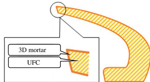
Figure 4. Layout of 3D mortar and UFC (Fully filled)
