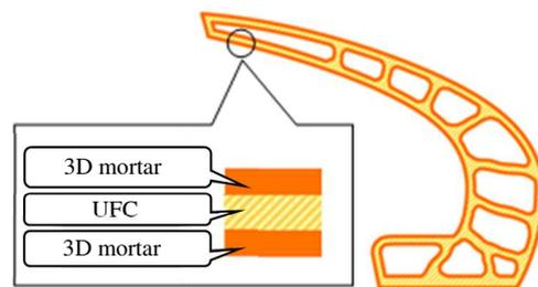
Figure 5. Layout of 3D mortar and UFC (Structurally rational)
