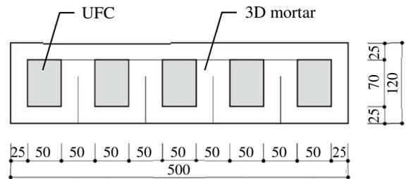
Figure 1. Cross section of the composite structure
