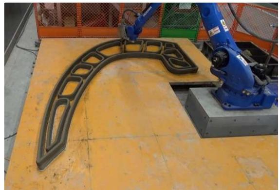
Photo 7. Printing of 3D mortar (at the start)
