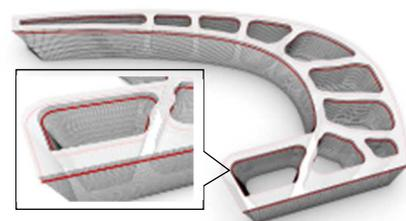
Figure 10. Automatic generation of the print path
