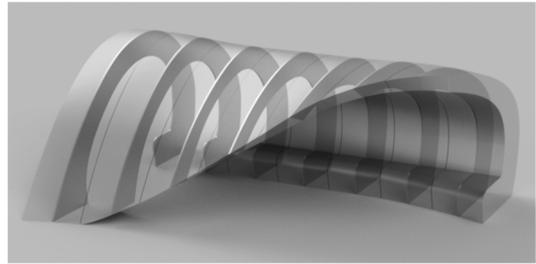
Figure 7. Sections to apply topology optimization
