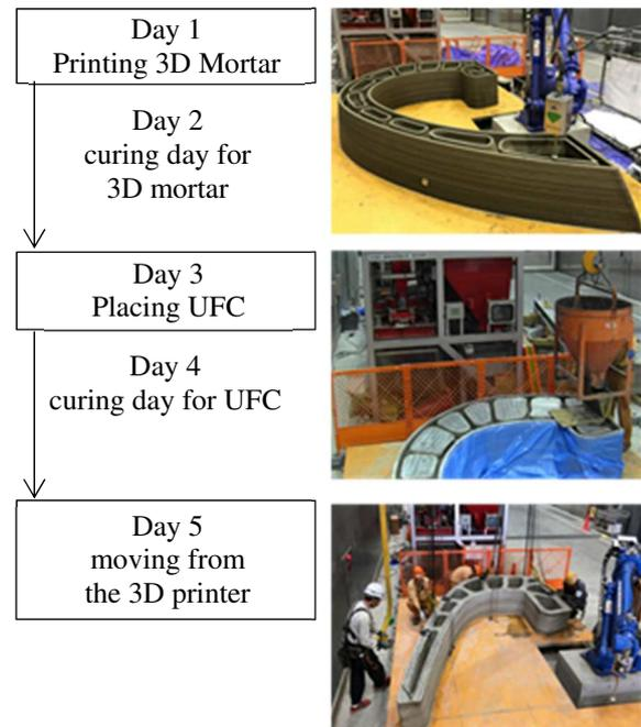
Figure 11. Manufacturing process of shell-shaped bench
