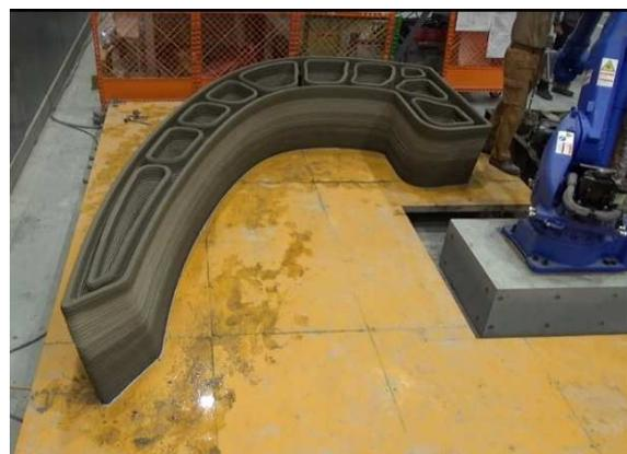
Photo 8. Printing of 3D mortar (at the finish)
