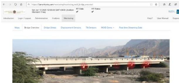
Figure 15. Bridge sensor's platform (location of sensors)
