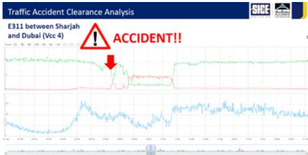
Figure 20. Traffic incidents detection from traffic live monitoring
