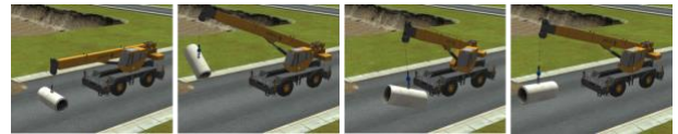
Figure 4. At first, the load suspended by the crane is intentionally shaken a certain amount. After a certain time, the operational agent reduces sway of a load suspended from a mobile boom crane.
