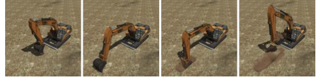
Figure 7. The agent operates only the bucket part. The agent scoops as much soil as possible in accordance with the movement of the excavator that follows a certain trajectory.
