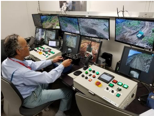
Figure 10. External remote control room in Aso-Ohashi area in which the number of operators is only one.
