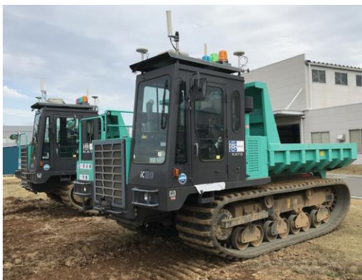
Figure 1. Two Crawler carriers for transporting earth and sand.
