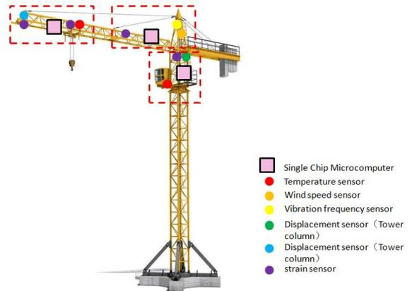
Figure 7. Diagram of the location of MCU
