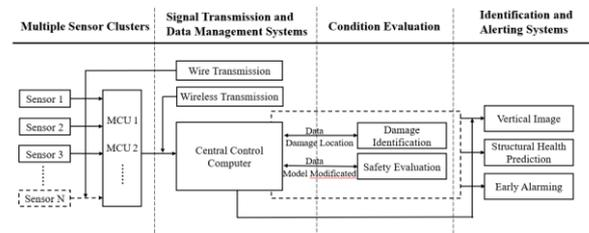
Figure 2. Workflow of safety monitoring system
