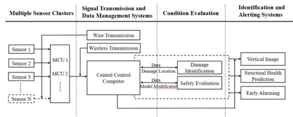
Figure 2. Workflow of safety monitoring system
