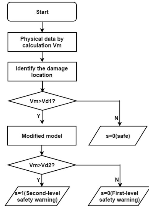
Figure 5. Workflow of condition evaluation
