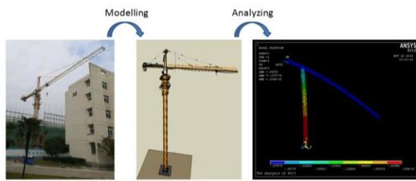
Figure 1. Data-driven modelling of tower cranes
