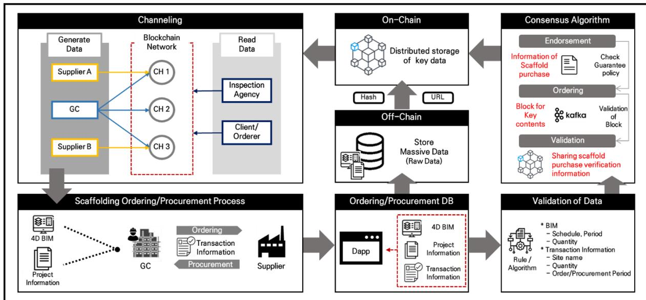
Figure 2. Blockchain-based scaffolding management process and key features
