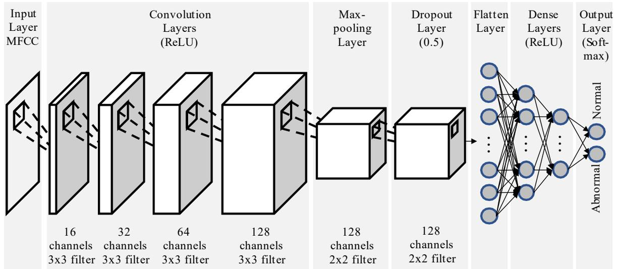
Figure 2. Detailed architecture of the convolutional neural network
