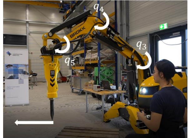
Figure 3. The task considered in this work: By moving the joints q_3, q_4 and q_5 with joysticks the operator tries to end-effector tip straight forward.
