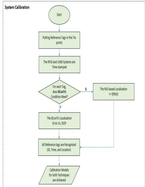
Figure 5. System calibration diagram.
