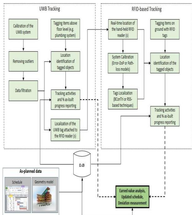
Figure 4. Conceptual overview of the location identification material tracking system.
