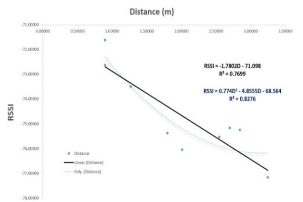
Figure 6. RFID system path-loss model.
