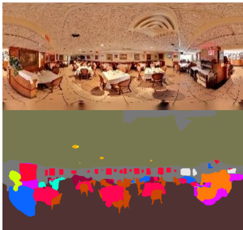
Figure 8. Sematic segmentation of an image from indoors. Top: original image; Bottom: segmented image, where each colour represents a different category of objects.
