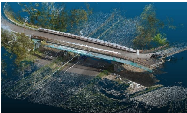
Figure 1. Three-dimensional point groups model of the whole bridge view
