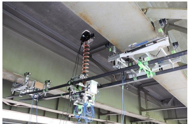
Figure 3. Flange-suspended type inspection robot Turrets
