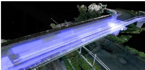
Figure 8. Superimposing three-dimensional points group data and CIM
