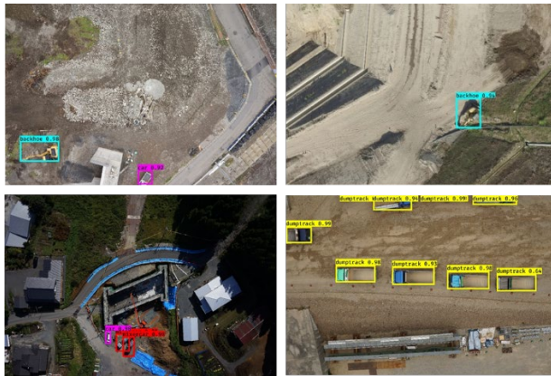
Figure 5. Example of construction machinery detection by YOLOv3
