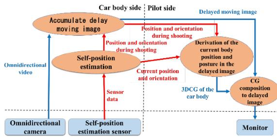
Figure 7. System Configuration
