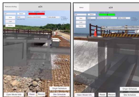
Figure 10. Excavation depth confirmation on the construction site.
