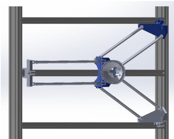
Figure 8. CAD PKM – designed for downscaled version
