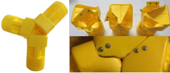
Figure 2. Development of the node from the unrecyclable plastic container using a combination of D2RP and traditional methods
