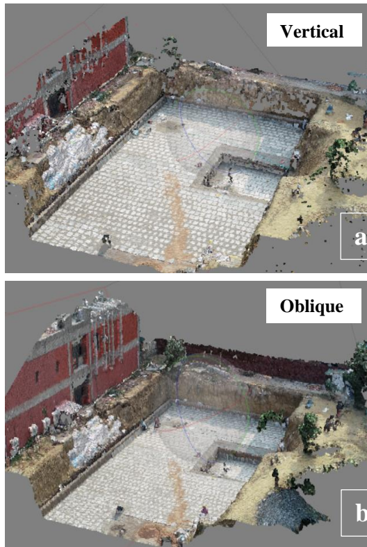
Figure 8. 3D point cloud model of the vertical and oblique images. 3D point cloud model shown in Figure 8 suggest models developed using oblique images to have more coverage and feature points. The number of data points generated were also high in case of oblique images as shown in table 1. The results are in agreement with observations by previous researchers where the angle between ground and the camera was found to significantly affects the density of point cloud generated [21, 22]. Aicardi et al. (2016) and Chen et al. (2017) recommend using an inclination angle of 0^\circ to 30^\circ for obtaining dense data clouds as the points density start decreasing for angles above 30^\circ .
