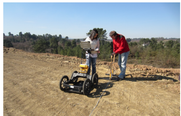
Fig.2. Data acquisition setup composed of the 200 MHz unshielded antenna.
