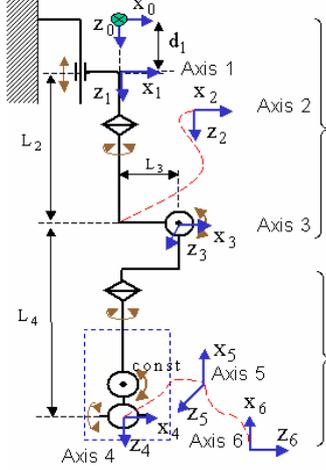
Figure 4. Kinematic analysis of the developed robot
