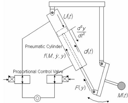
Figure 6. Schematic of pneumatic system (serial axis 3)
