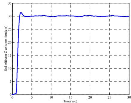
Figure 8. Suspending of end-effector position
