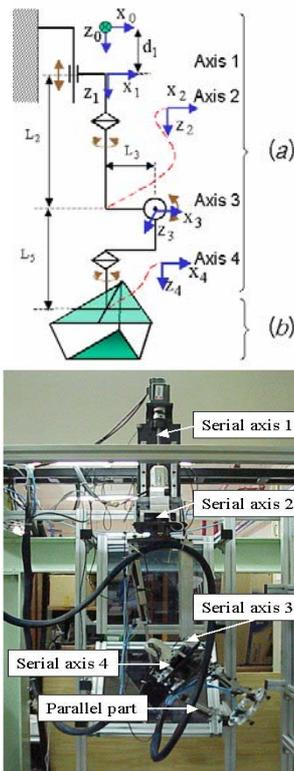
Figure 1. Serial-parallel hybrid type robot model
