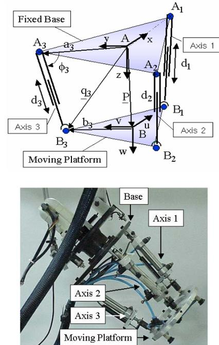
Figure 2. Parallel part of the developed robot
