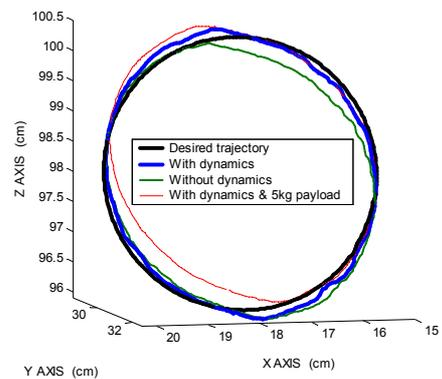
Figure 9. End-effector path control
