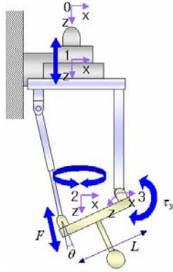
(a) Schematic of the discrete model
