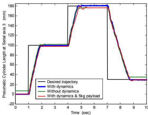
Figure 7. Step position response of the serial axis 3
