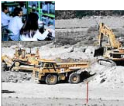
Fig.3 Actual use of remote controlled earth moving machines at Mt. Unzen-Fugen disaster site.
