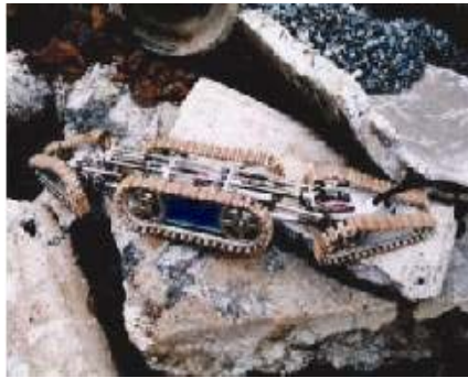
Fig.5 Snake-Type Robot "SORYU" developed by Tokyo Institute of Technology.
