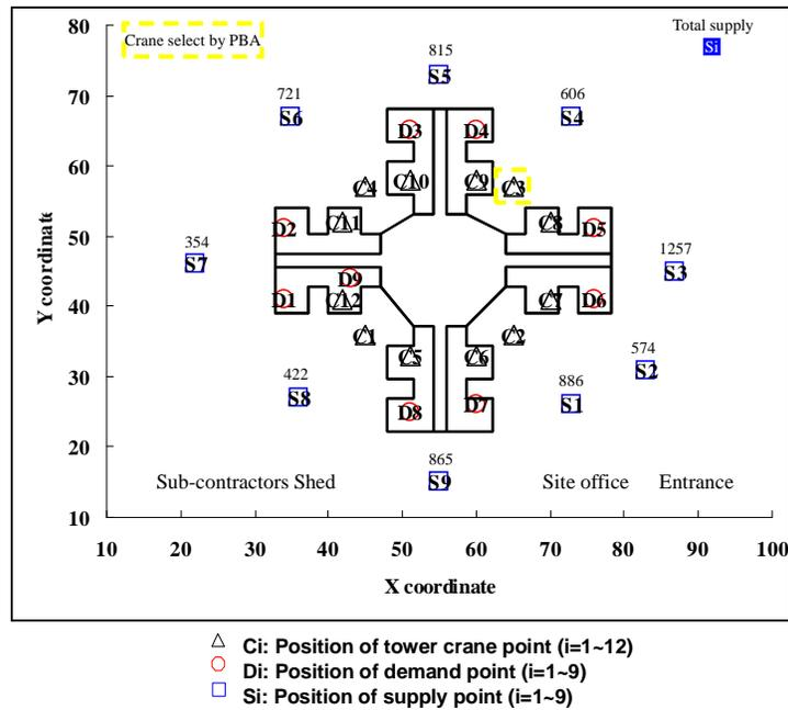
Figure 4 – PBA best single tower crane layout design
