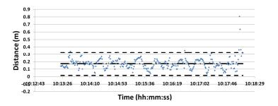
(b) Distances between the two tags on the excavator body
