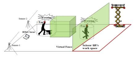
Figure 2 - Concept of sending warnings to workers on foot
