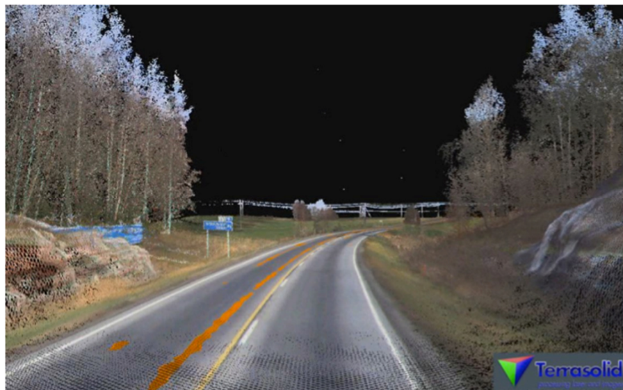
Figure 2. An example of the analyzed and modelled 3-D point cloud. The geometric pits and deviations have been coloured (Terrasolid). There were observed many new useful possibilities to detect and model useful information for road improvements from the point cloud.
