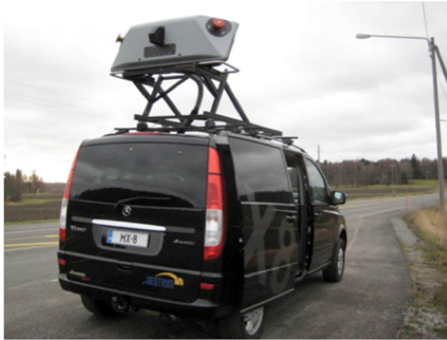
Figure 1. Trimble MX8 mobile mapping system was used for the laser scanning and photogrammetric measurements. As driving speeds in the pilots Mt116, Kt51 and Vt6, the 50-65 km/h, 40-50 km/h and 50-70 km/h, were used, respectively. The speeds were varied due to different road, traffic and environment conditions.
