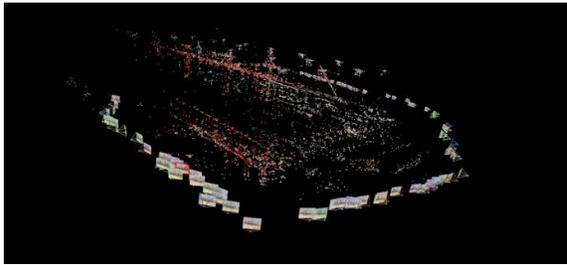
Figure 14. Point cloud model reconstructed from 100 images with camera frusta
