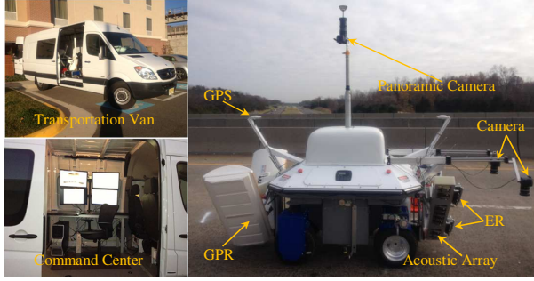
Fig. 1. The bridge robotic inspection system with the command center built in the transportation van.
