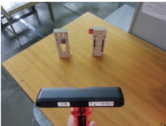
Figure 6. 3D connector shape registration using depthmap of Xtion Pro Live
