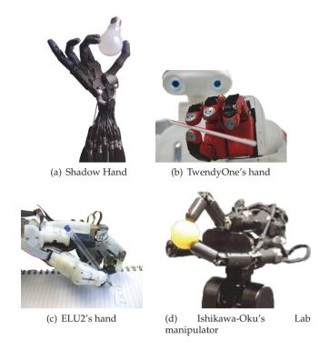
Fig. 3. Samples of different state of the art manipulators.
