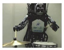
Fig. 8. Two-handed drumming using the Sarcos CB-i humanoid robot.
