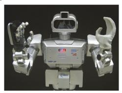
Fig. 2. Humanoid HRP3P with multi-fingered hand
