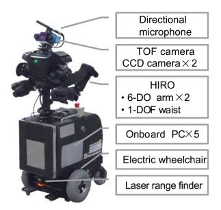
Fig. 6. The robot platform "DiGORO".
