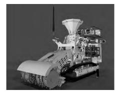
The bulk cutter ROV is designed to segregate material collected from the seafloor.
