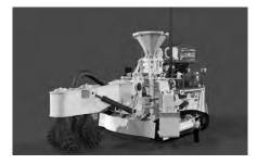
The 250-tonne auxiliary cutter will clear the way for the other ROVs to operate. (All images in this article courtesy Nautilus Minerals and SMD.)
