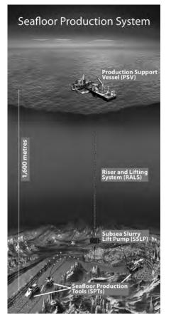
Graphic rendering of the oceanmining system designed by Nautilus in collaboration with SMD.
