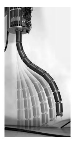
A composite photo of OC Robotics' Explorer snake robot reveals its flexibility, an asset when the device operates in cramped quarters. (Photo Courtesy OC Robotics.)
