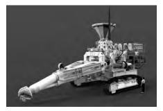
The collecting machine ROV will pump material in slurry form to the ship.
