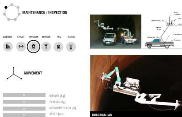
Figure 5. First Survey: Tunnel inspection robot developed by Universidad Carlos III de Madrid.
