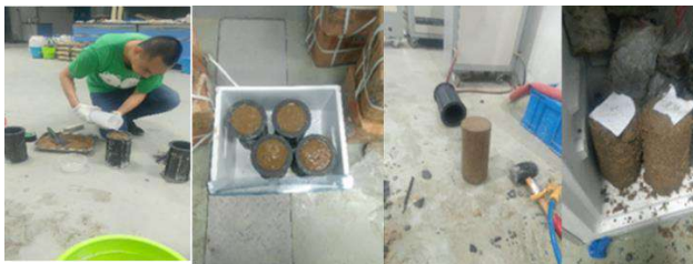
Figure 2. Preparation of frozen soil specimen
