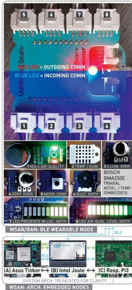
Figure 2. BLE Wearable Node as WSN / BAN, Features.
