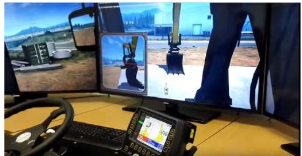
Figure 1. Test simulator (Tenstar) integrated to Leica's 3D machine control system to practice the use of excavator.
