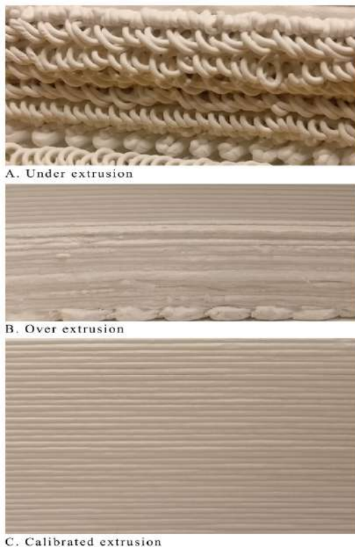
Figure 4. Results of 3D printing speed calibration. A. Under extrusion speed, B. Over extrusion speed, C. Calibrated extrusion speed
