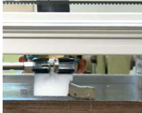
Fig. 4: Concrete technological extrusion trials on a scale of 1: 5
