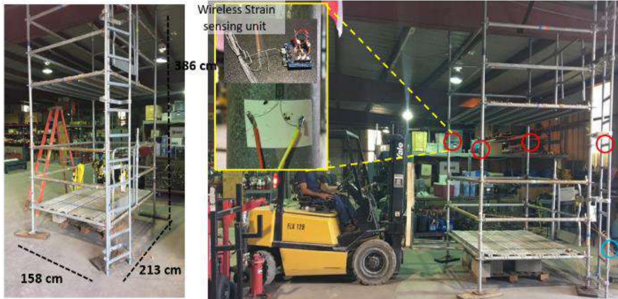
Figure 4 Experimental setup with a one-bay scaffold
