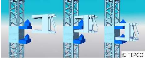
Figure 2. Mating Connection Mechanism
