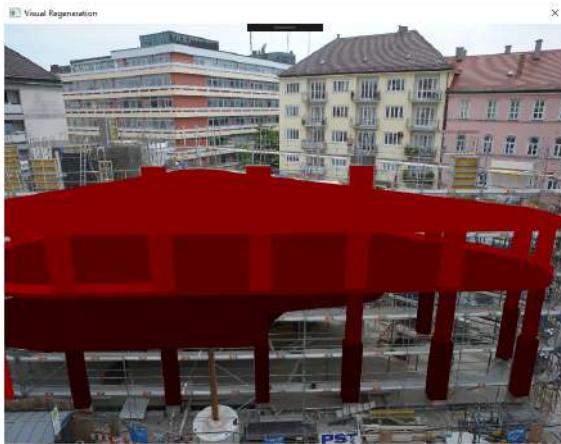
Figure 6. Using re-projection methodology for model rendering based on the Painter's Algorithm and 4D semantic information
