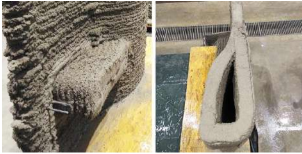
Figure 11. Wall produced with Shotcrete 3D Printing; Detail of the console, with 2 reinforcement bars left blank (left); top view of the wall (right)
