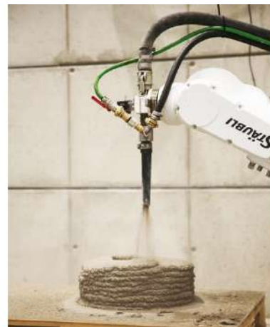
Figure 8. Application process of the new developed Shotcrete 3D Printing technology
