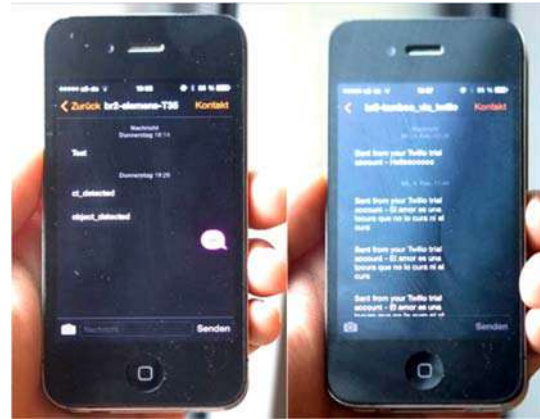
Figure 4. Left: SMS via WiFi (Twilio®). Right: SMS via Siemens T35 GSM module.
