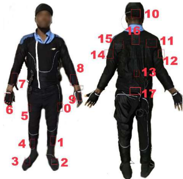
Figure 4. Inertia 3DSuit infrastructure showing the location of the IMU sensors.
