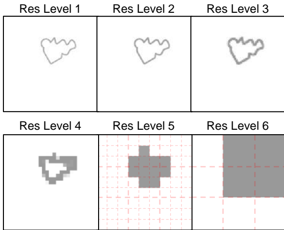
Figure 3. Model lookup tables at various resolution levels for an arbitrarily shaped object
