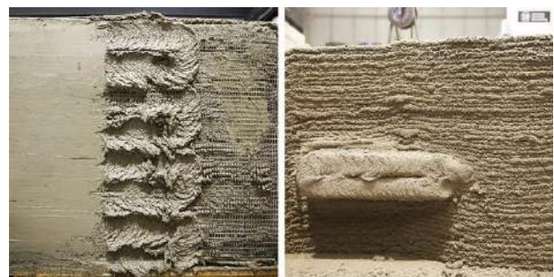
Figure 10. Wall produced with Shotcrete 3D Printing; backside smoothed and with implemented textile reinforcement (left); frontside with steel reinforced sprayed console (right)
