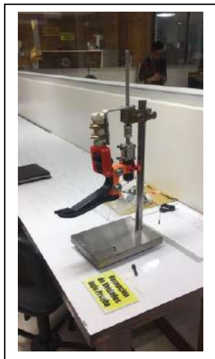
Figure 9. Functional model of the sole with the electric actuator attached.
