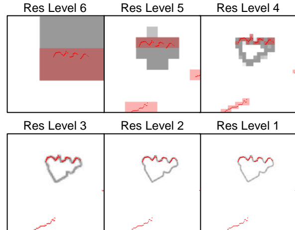
Figure 4. Example GRCSM search process showing the best fit results at each resolution level leading to the final fit result
