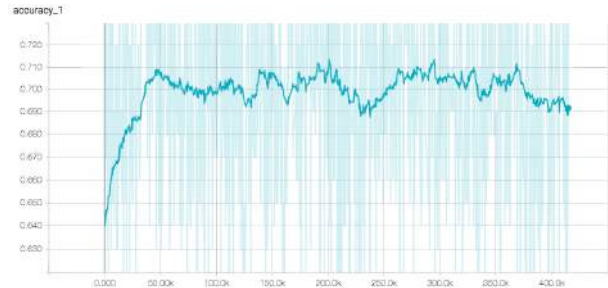
Figure 2. Accuracy (y-axis) changes according to the number of trainings (x-axis). Average accuracy (thick line) first rises dramatically but then hardly changes after the training time exceeds 50,000.
