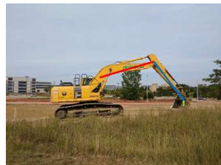
Figure 1. Excavator pose is determined by identifying its joints and components.
