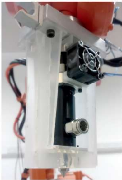
Figure 2. The industrial extruder with the supportive system mounded on the robotic arm
