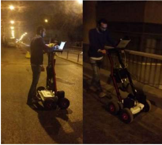
Figure 3: GPR data collection for El-Kobba bridge deck
