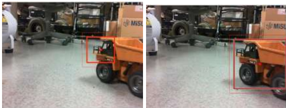
Figure 11. The result of improved template matching method at the big turning
