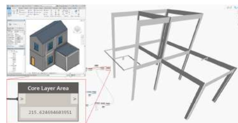
Figure 4. The surfaces of the walls that intersect with columns, beams, and floors are shown in Dynamo. The net core layer area of the wall is calculated.
