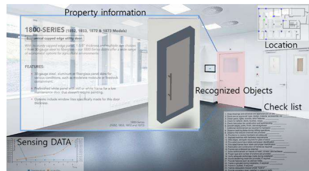
Figure 6. Example of AR-based SFM system UI
