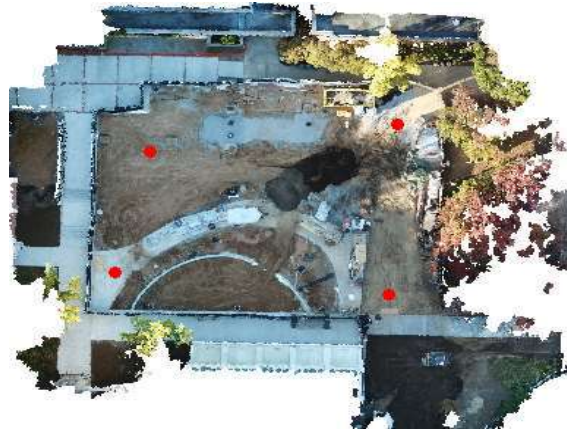
Figure 6. Identified scan locations from the scan planning simulation with UAV's point cloud (top view)
