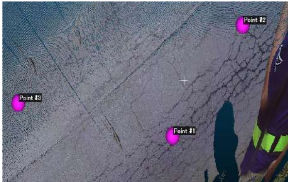
Figure 11. Repair information linked with three-dimensional point cloud data
