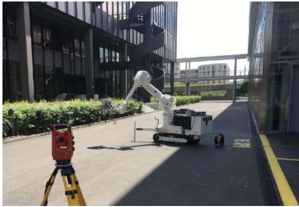
Figure 1. Setup exploring the use of an external measuring system in the form of a robotic total station for localization.
