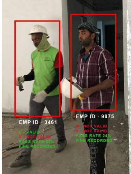
Figure 6. Face recognition using smart hard hat
