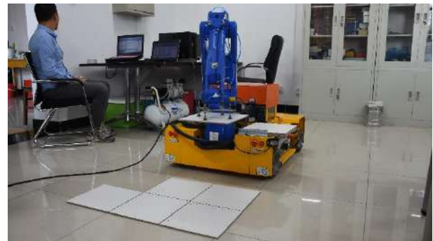
Figure 11. Measuring and positioning test of robotic floor-tiling
