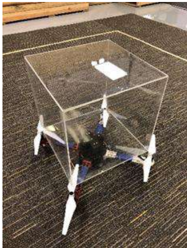
Figure 2. Prototype UAV with an acrylic cube box (a module)
