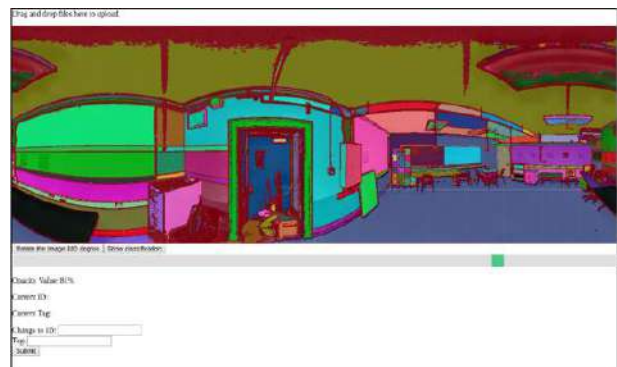
Figure 5. Panoramic image view with colormap overlay representing the instance segmentation results obtained using Norvana algorithm
