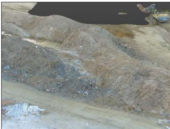
Figure 7. Digital terrain model generated using the proposed method
