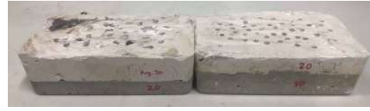
Figure 5. Concrete lab samples - 20mm gypsum layer with no aggregates (right) and 30mm gypsum layer with 10mm aggregates (left).
