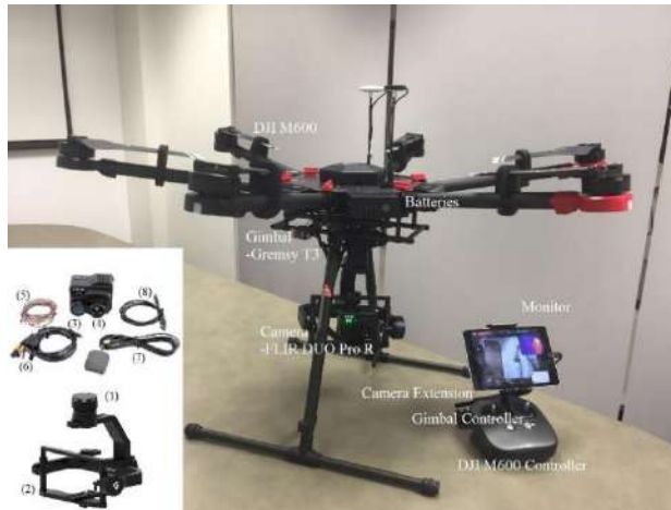
(1) Gimbal - Connection to DJI M600; (2) Gimbal - Frame for Camera; (3) FLIR DUO Pro R - Visible Lens Barrel; (4) FLIR DUO Pro R - IR Lens Barrel; (5) FLIR DUO Pro R - Electric Wires; (6) FLIR DUO Pro R - Integration Cable; (7) FLIR DUO Pro R - GPS Antenna Cable; (8) FLIR DUO Pro R - USB Cable.
