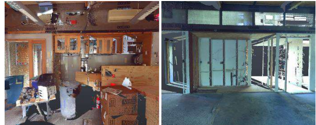
Figure 7. Metal studs behind the kitchen region are invisible in Scan 1 (left) but become visible in Scan 2 (right)
