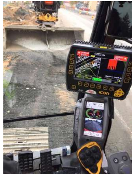
Figure 2. Commercial example: the Leica iCON iXE3 Copilot.
