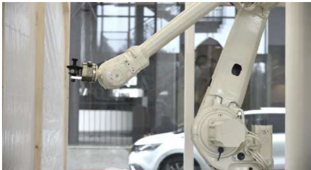
Figure 3. Reflector prism mounted on the end-effector of IF.
