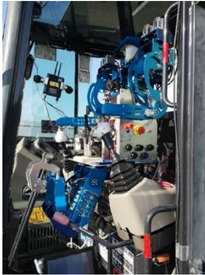
Figure 4. Research project in Japan by Kanamoto Ltd, on a movable humanoid remote robot for remote control.
