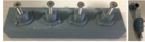
Figure 5. (Left) Assembled electrode arrangement. (Right) Electrode with spring mechanism.
