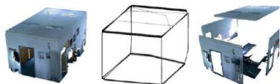
Figure 5. Point cloud segmentation for planar segments. Left: Input point cloud. Center: Wireframe model. Right: Segmented point cloud.
