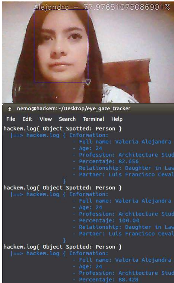
Figure 5. Recognition of a familiar face and corresponding output of associated information pertaining to the identified person.
