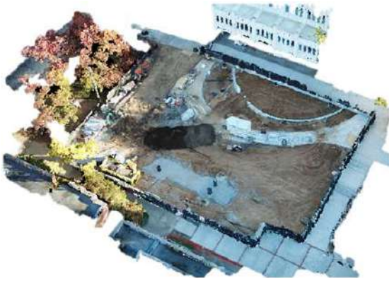
Figure 3. UAV-generated 3D point cloud map of the construction site using image data
