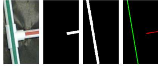
Figure 5. Ground truth pose generation. From left to right: Warped image, detected red mask, detected green mask, green and red tape skeletons estimation. The pose of corresponding objects can be calculated according to the skeleton of color tapes.
