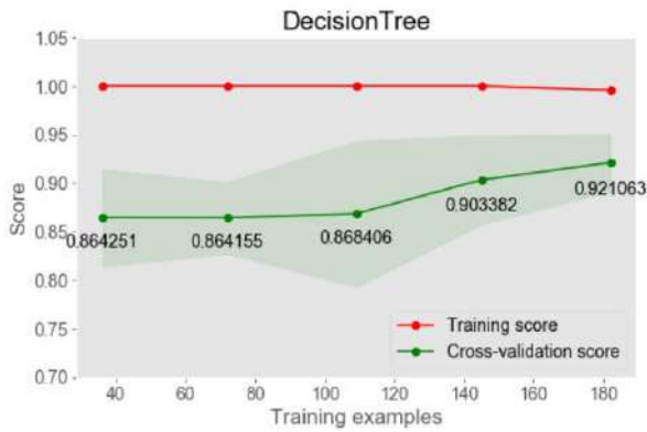
Figure 5. The learning curves of the classifier of a decision tree with a maximum depth of 6
