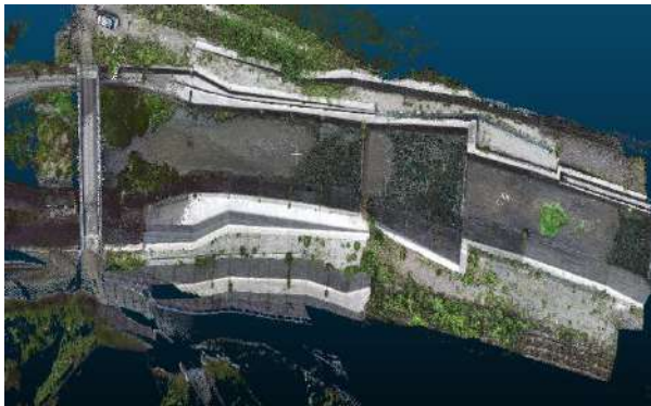
Figure 7. Data fusion of terrestrial laser scanning and UAV on a bridge
