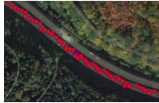
Figure 3. Visualization of the reversing points close to the paver from a real world example.
