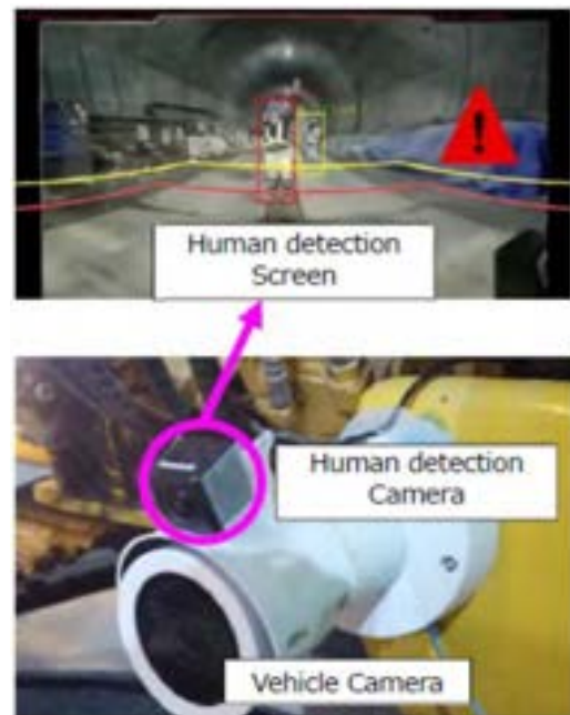
Figure 6. Human body detection camera (Above: Detected human body)
