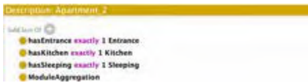
Figure 2. Composition constraint to define a three-module apartment
