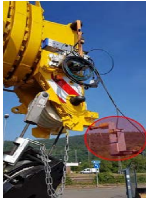
Figure 1. Crane load-view camera circled in red.
