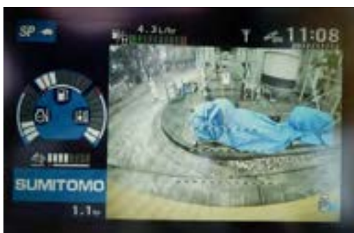
Figure 12. Examples of not being a person, but recognizing a person as a person
