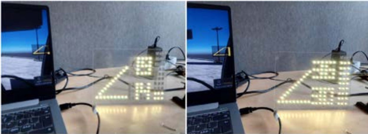
Figure 6. The examples that show the integration between the virtual transparent display and its physical counterpart. The examples were made when the virtual mobile crane was using the 4.8-tonne counterweight and lifting a 1-tonne load. The left image shows the boom length was 19 m, the load radius was 14 m, and the lifting capacity was 20% used. The right image shows that the boom length was 36 m, the load radius was 30 m, and the lifting capacity was 90% used.
