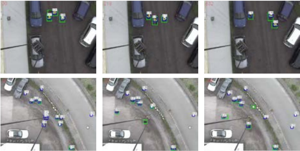
Figure 6. Predicted results of trial BL on the test sequence R1 in the first row (frame 30, 219, 632) and R2 in the second row (frame 40, 297, 348). The blue bounding box is the detected target with confidence score label while the green box is groundtruth.
