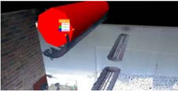
Figure 3. An example of a traditional QA/QC workflow, where deviations are eyeballed in software and measurements are prone to human error.
