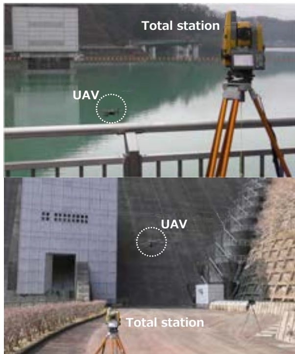
Figure 6. The flying UAV and tracking by the total station (Dam-1). The above image shows the tracking from above and the image below shows tracking from below.
