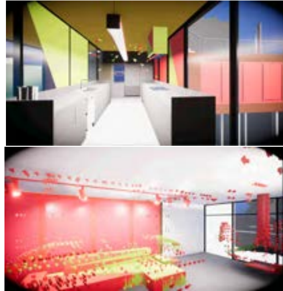
Figure 6. Animated Arrows visualisation. Top image shows the visualisation with a UGR > 24 whereas the bottom image contains a UGR threshold of > 0
