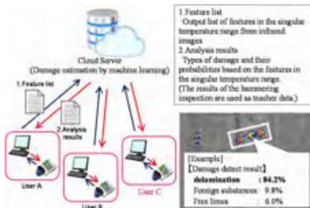
Figure 8. Automatic detect system using a cloud server
