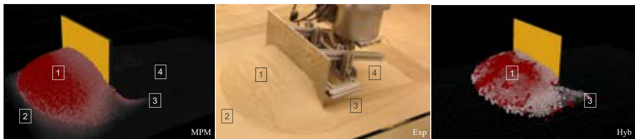
Figure 8. Geometries of soil deformations in MPM, Hybrid, and experiment for 5-cm depth. Four visual criteria are emphasized for comparison.
