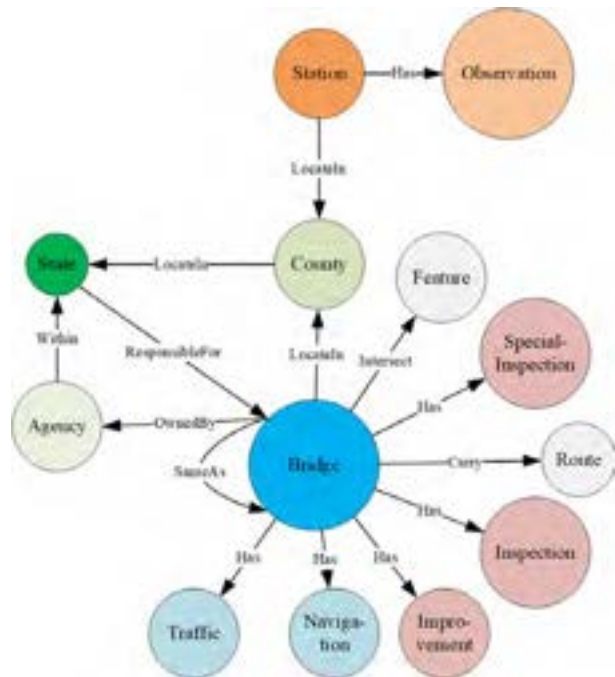
Figure 2. Concept graph model for bridge management
