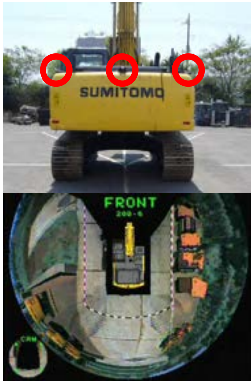
Figure 2. An example of a three-camera arrangement and image composition
