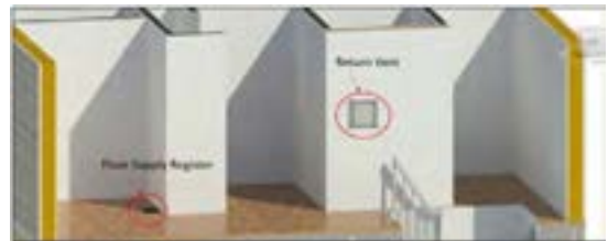
Figure 5. 3D rendering of a floor register and a side wall return vent in Revit (displacement ventilation)
