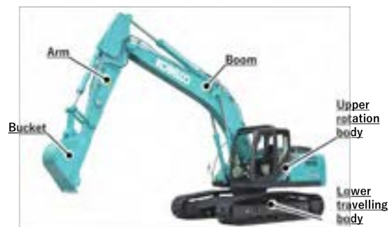
Figure 1. Hydraulic excavator components
