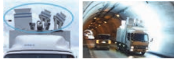
Figure7. Installation and Measurement of Internal Defect Radar Antenna
