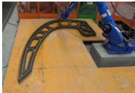
Photo 7. Printing of 3D mortar (at the start)
