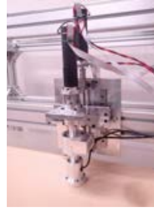
Figure 4. Small-diameter plate load test equipment
