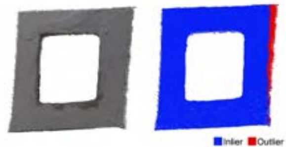
Figure 6. Task 1 results. Left: RGB point cloud captured by Kinect. Right: visualization of Layer Deviation between scanning point cloud and CAD file. Signed error is color coded from red (positive) to blue (negative).
