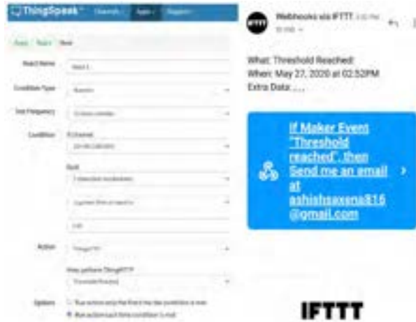
Figure 8. Setting up Threshold in ThingSpeak & receiving a warning from IFTTT
