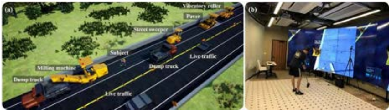
Figure 1. Experimental environment: (a) the landscape of the immersive virtual road construction environment, (b) the Building Information Modeling-Computer Aided Virtual Environment (BIM-CAVE)
