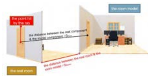
Figure 8. Room model distance before rotating \Delta Q is not equivalent to the sub-component distance.
