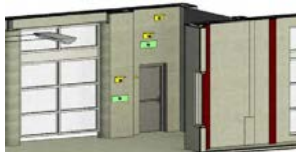
Figure 2. Closeup within the parametric model of experiment room showing embed placement
