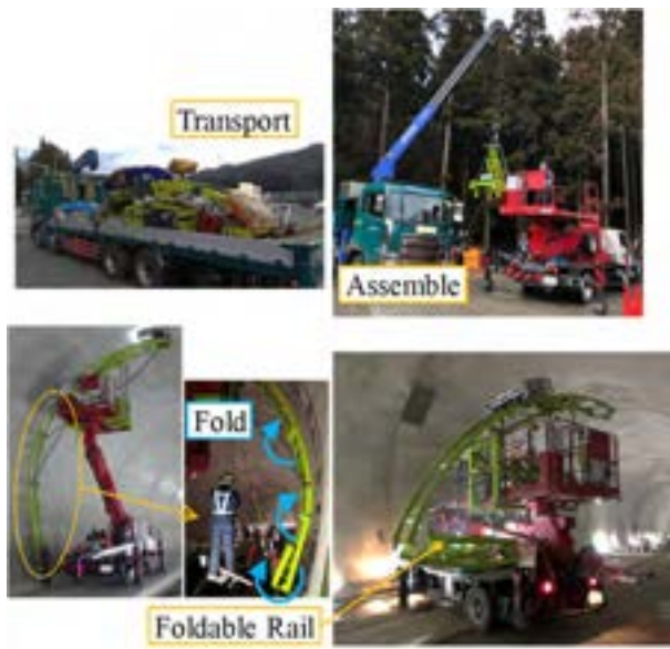
Figure 8. System Transport, Assemble and Foldable Rail of Half-Section-System
