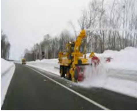
Figure-1. Snow and ice countermeasure work on the expressway (snow blowing work)
