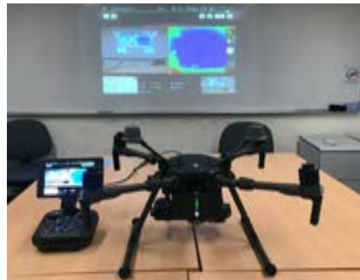
Figure 5. DJI Matrice 210 V2 RTK used for the study
