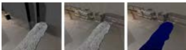
Figure 14. Water particles generation by NVIDIA FleX for Unity on 3D measurement model
