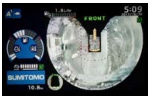
Figure 11. Display of recognition results on the composite image
