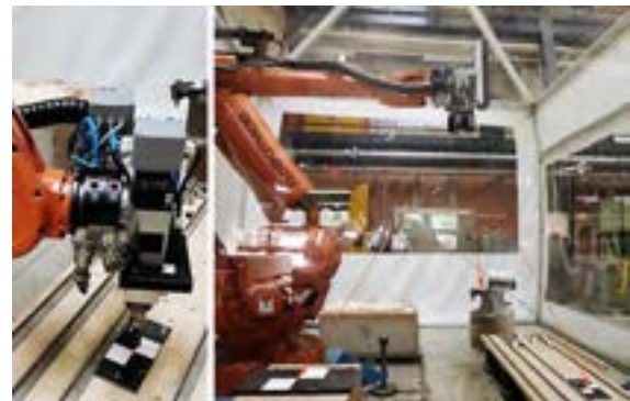
Figure 8. Targets are measured by a sharp-tool and captured by the laser-scanner.
