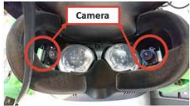
Figure 4. Two cameras installed inside the head-mounted display
