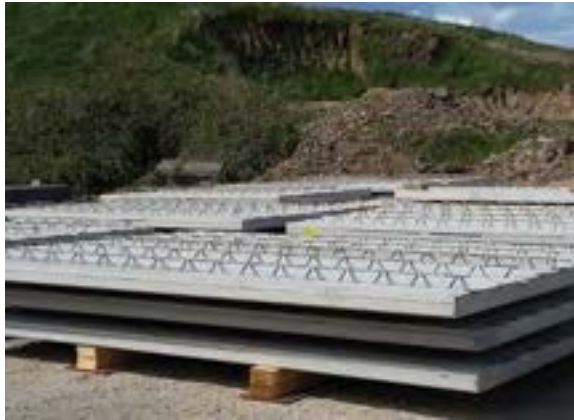
Figure 6. Shear key as Lifting Hook in Lattice Girder
