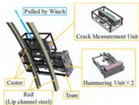
Figure 5. Mechanism of Inspection Device Transfer
