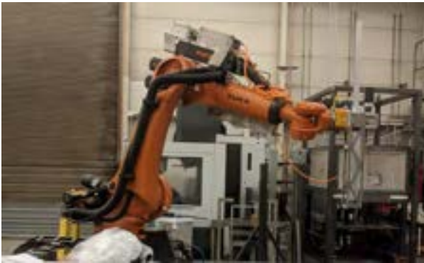
Figure 5. The KUKA KR120 robotic arm for the physical robot module.
