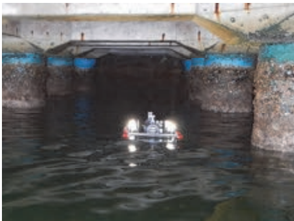
c) Automatic shooting underside of pier superstructure
