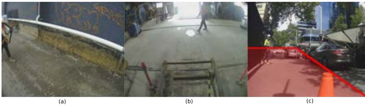
Figure 5. Example TBS viewpoint images from each of the test datasets as outlined in Section 4.1, illustrating the visual variance tested. (a) is mounted on a vehicle in an outdoor environment, (b) on moving machinery indoors, and (c) on stationary infrastructure on road. Example (c) illustrates how a user defined exclusion zone (shown in red) is displayed in the UI, as described in Section 3.4.
