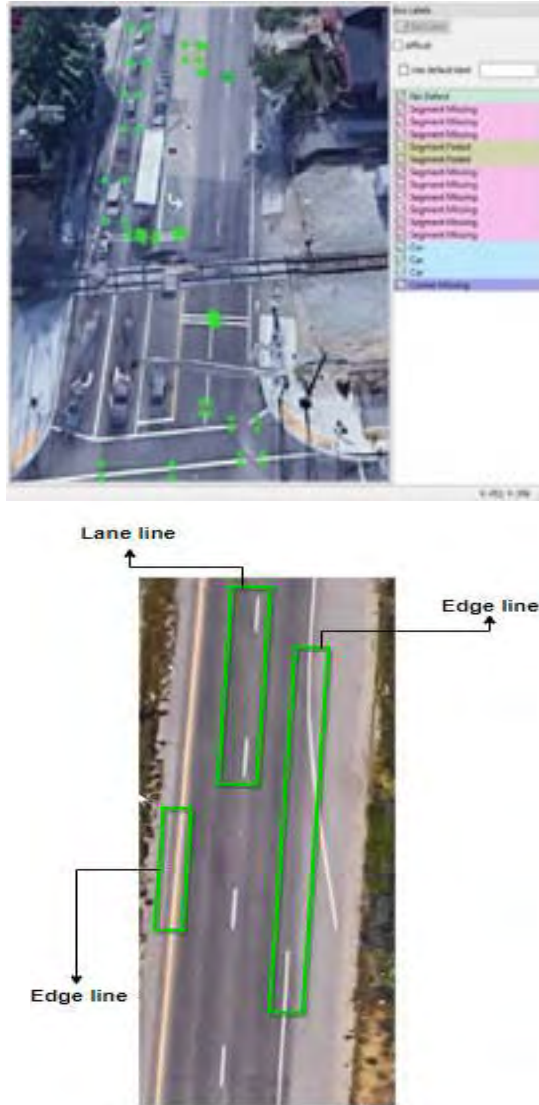
Figure 2. Pavement Marking Annotation and Data Preparation for Model Training
