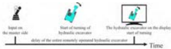
Figure 1. Delay occurred in teleoperated excavators
