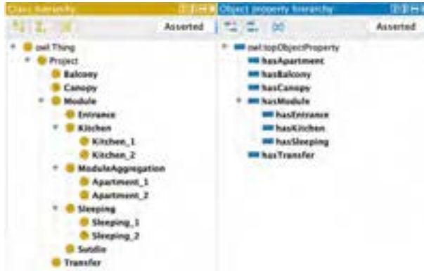
Figure 1. Class hierarchy and object property hierarchy of the modular building
