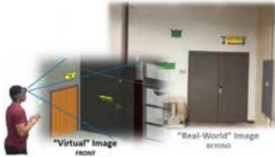
Figure 6. Framework of inspecting embeds using AR
