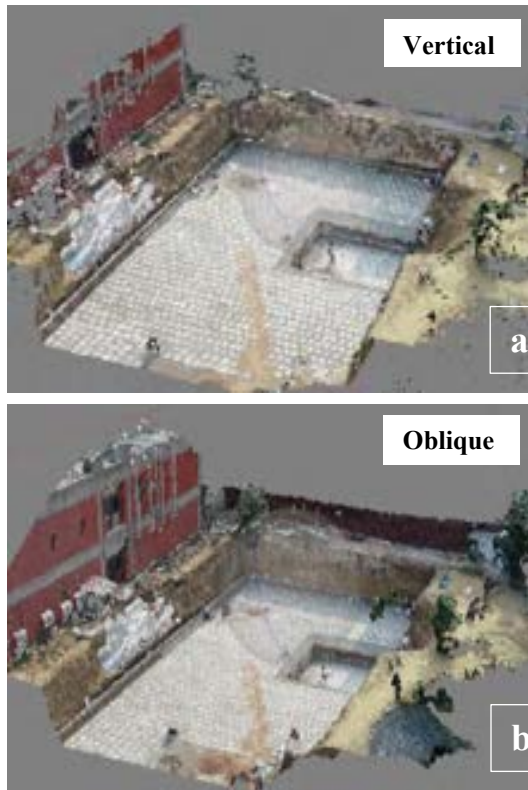
Figure 8. 3D point cloud model of the vertical and oblique images. 3D point cloud model shown in Figure 8 suggests models developed using oblique images to have more coverage and feature points. The number of data points generated were also high in case of oblique images as shown in table 1. The results are in agreement with observations by previous researchers where the angle between ground and the camera was found to significantly affect the density of point cloud generated [21, 22]. Aicardi et al. (2016) and Chen et al. (2017) recommend using an inclination angle of 0^\circ to 30^\circ for obtaining dense data clouds as the points density start decreasing for angles above 30^\circ .
