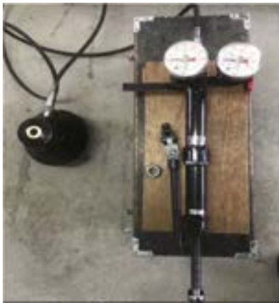
Figure 8. Manual Pull-off adhesion tester.
