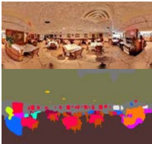
Figure 8. Semantic segmentation of an image from indoors. Top: original image; Bottom: segmented image, where each colour represents a different category of objects.
