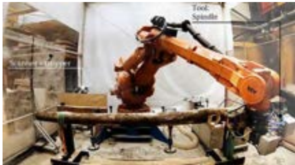
Figure 5. Cutting process using spindle and milling while the scanner and gripper is removed.
