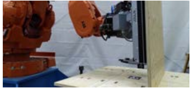
Figure 13. Insertion of a laminated veneer lumber (LVL) panel with the visual feedback loop.
