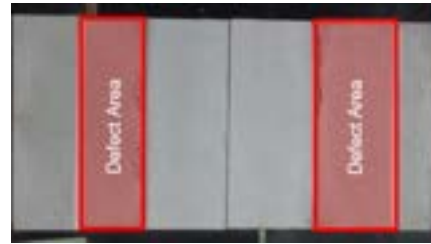
(b) Case 2: dual delaminations.
