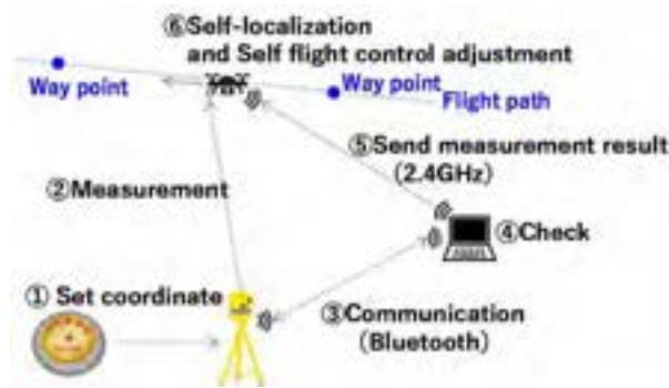
Figure 3. Image of the proposed UAV navigation system using the total station.
