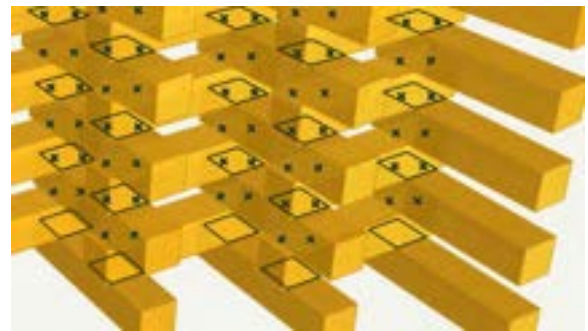
Figure 4. Geometry nailing points and gluing range
