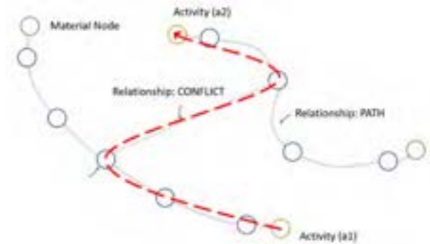
Figure 4. Example for finding colliding routes by traversing the graph
