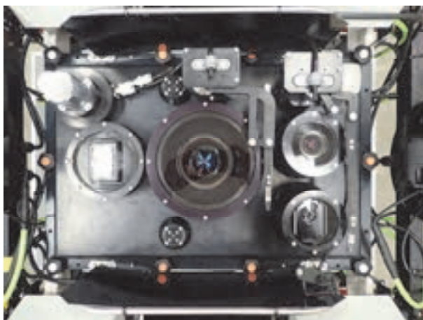
b) Camera system with glass surface cleaning function
