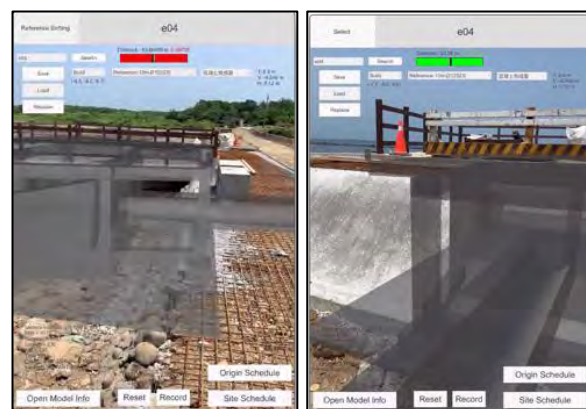
Figure 10. Excavation depth confirmation on the construction site.
