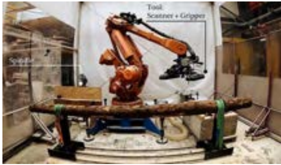
Figure 4. Laser scanner is positioned on a vacuum gripper. When the scan is finished the tool is automatically changed to the spindle
