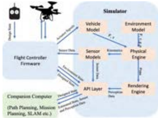
Figure 2. AirSim simulator architecture (reproduced from [28])
