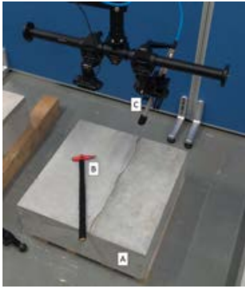
Figure 3. The experimental setup in laboratory conditions with (A) a concrete test block containing a simulated defect, (B) a hammer and (C) a microphone to record the hammering sound.
