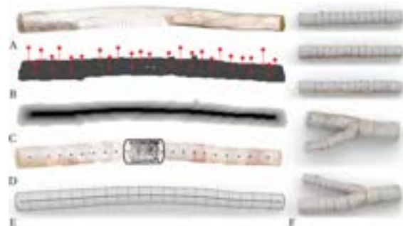
Figure 11. A - PointCloud, B - Projection, C - 2D Thinning, D - Cylinder-fit, E - Radial parameters, F - Application in straight, curved and forked trees.
