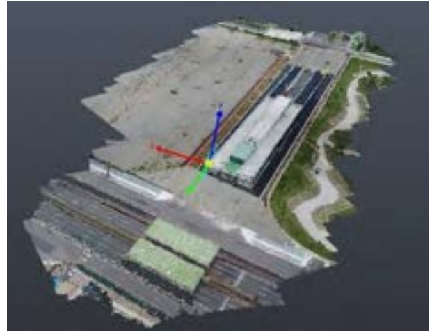
Figure 9. Updating the origin of the point cloud model
