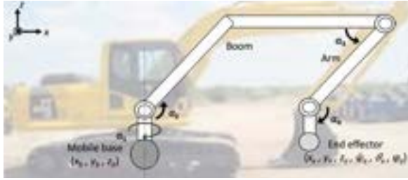
(a) Model parameters for excavator joint configuration
