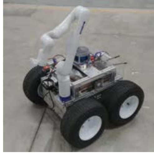
Figure 5. Mobile robotic platform used in our experiments, here with an additional arm mounted.
