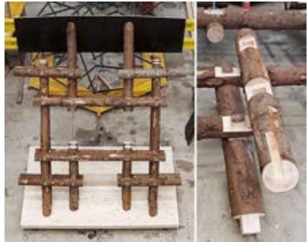
Figure 13. First prototype in small radius round-wood made using the applied methodology.
