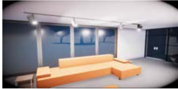
Figure 1. This image presents the standard HDRP Lighting Visualisation: which is a realistic representation of Glare within the scene. Lights are set to 800 lumens and a 3 meter range.
