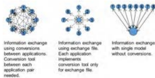
Figure 1. The basic differences for the needed conversions with the different data exchange methods. With application to application, the total number of conversions is the largest, whereas with a single shared model no conversions are made.
