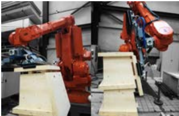
Figure 9. Assembly of 13 non-orthogonal timber panels without using the visual feedback loop.
