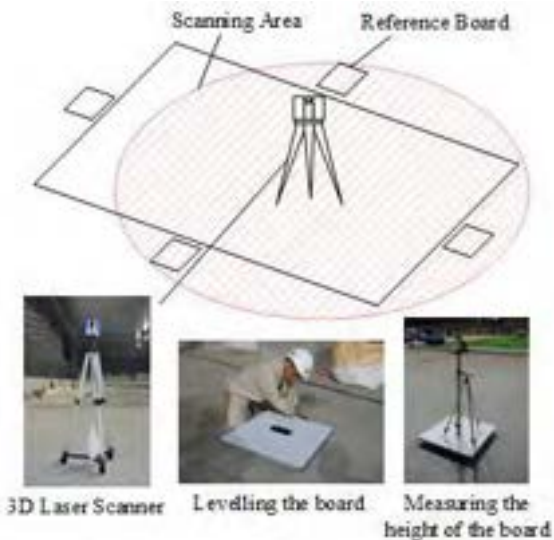
Figure 12. Proposed measurement method
