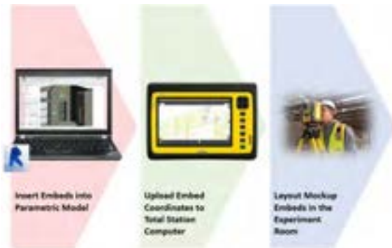
Figure 3. Workflow for migrating parametric model information to a total station for embed layout
