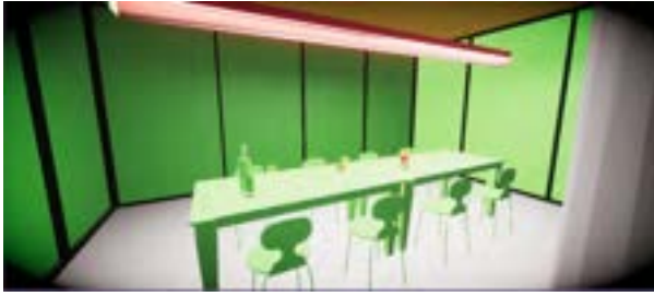
Figure 2. This image presents the heatmap Lighting Visualisation: which generates a three-dimensional heatmap to represent the amount of Glare within the scene. Lights are set to 800 lumens and a 4 meter range.
