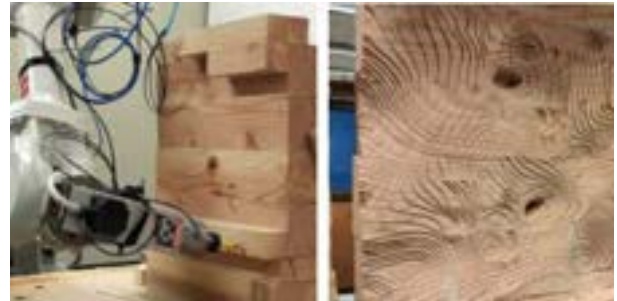
Figure 4. Panels with integrated acoustic and structural performance robotically produced at AUAS
