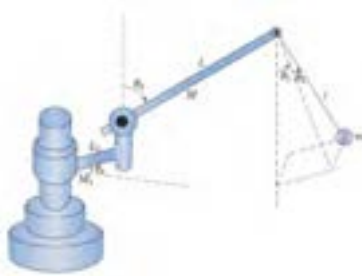
Figure 1. Model of an underactuated boom crane system. [20]
