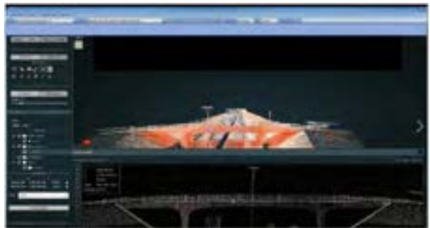
Fig 13. 3D model from LiDAR data. Creation of cross sections for post analysis in structural analysis
