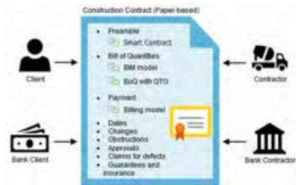
Figure 3. Integration of a smart contract into a construction contract
