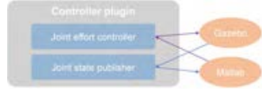
Figure 4. The framework structure of the simulation. The simulation is implemented in Gazebo. The controller is designed in Matlab. Using ROS communication mechanism, Matlab receives the current joint states from Gazebo, determines the joint efforts and sends them to Gazebo to achieve the final movement.
