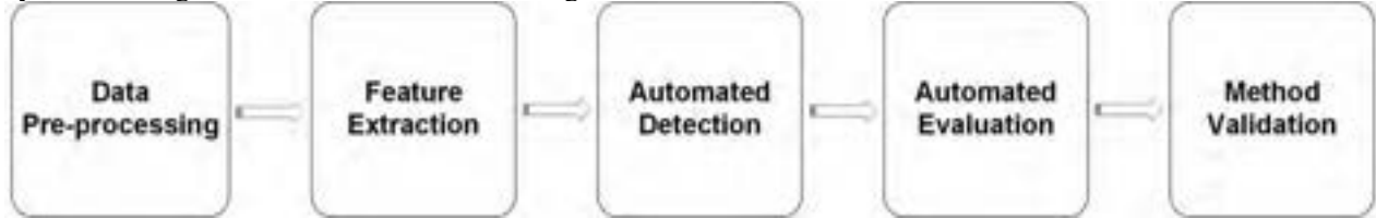
Figure 1. Main modules of the developed spalling detection model
