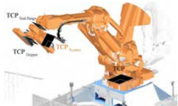
Figure 3. A laser scanner is mounted on a robot vacuum gripper and the TCP_{Scanner} is not known.
