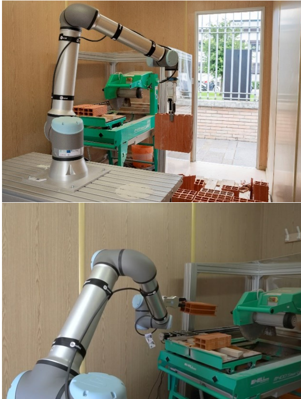
Figure 7 a/b: Automated brick cutting system
