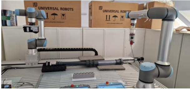
Figure 6. Full setup at home position. UR10e robotic arm outfitted with a stoneflower3D clay extruder on the right. And on the left a UR5e on a SlideKit linear axis outfitted with a Gocator 2330 laser profiler.
