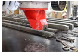
Figure 9. ProfiCarb process and view of the nozzle with 6 yarns [17, 29].
