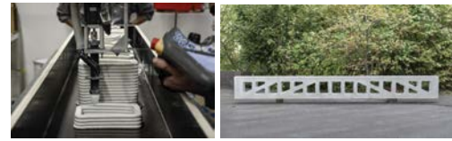
Figure 3. Prototype of an optimized reinforced concrete beam with printed formworks [23].
