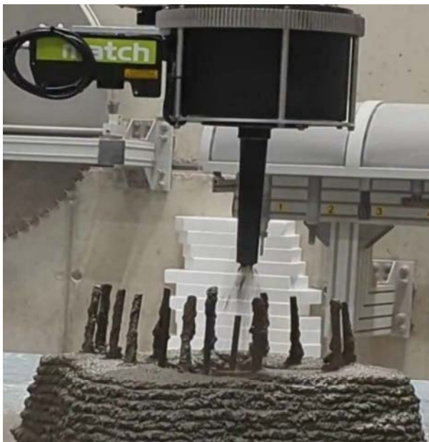
Figure 1. Shotcrete 3D Printing (SC3DP) at the DBFL of the ITE TU Braunschweig including short reinforcement bar insertion, as proposed by Dörrie et al. [7], and a 2D laser profiler running ahead of the printing nozzle. The goal of our paper is the detection of the depicted type of reinforcement elements.
