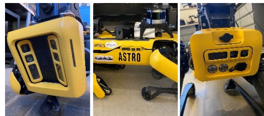
Figure 3. Front, side, and rear sensors and wide-angle cameras
