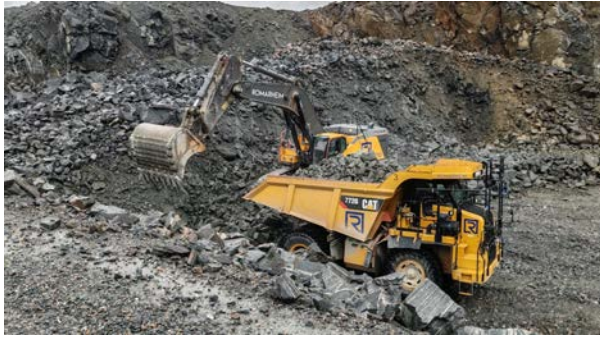
Figure 5. Autonomous dump truck at loading point.[25]
