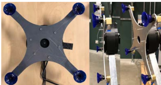
Figure 11. Pneumatic Components Assembly. A Physical Representation of the Implementation of the Pneumatic System as Depicted in Figure 7.
