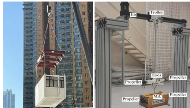
(a) Demonstration of connection between hook and MiC (b) The self-built 2-D overhead crane model
