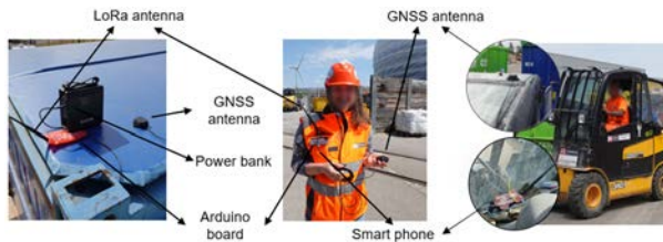
Figure 5. Setup of RTK-GNSS system on pedestrian workers and equipment.
