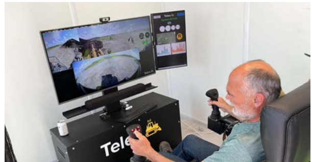
Figure 4. Control booth of retrofit remote control system.[22]
