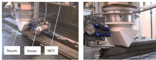
Figure 8. MCF nozzle with motorized routing of reinforcement under the extruded strand [27].
