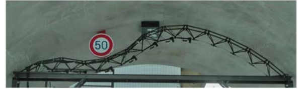
Figure 12 Shape control of guide frame avoiding obstacles in model tunnel
